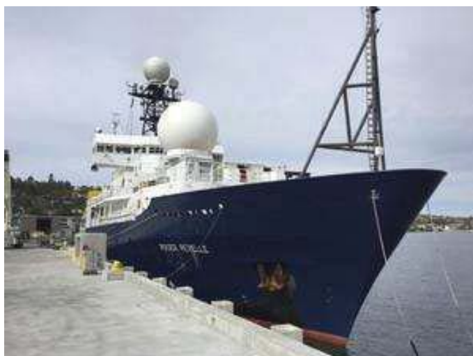
Photo of SEA-POL mounted on the 02 deck of the R/V Roger Revelle in San Diego before departing on the cruise.
