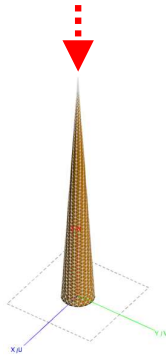
Figure 7. Geometry of the PEC cone scatterer with multiscale mesh, where the ratio of the longest to the shortest mesh edge is 228.5.
