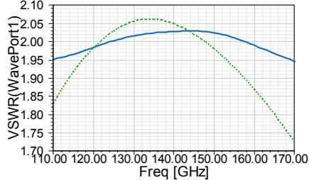
**Figure 5.** Simulation results of the mismatch waveguide with nominal VSWR 2.0 with different method (the dotted line is the traditional design, and the solid line is the new design)
