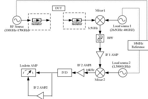
**Figure 8.** Block diagram of the attenuation measurement system
