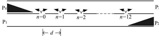
**Figure 6.** The internal structure of the attenuator.
