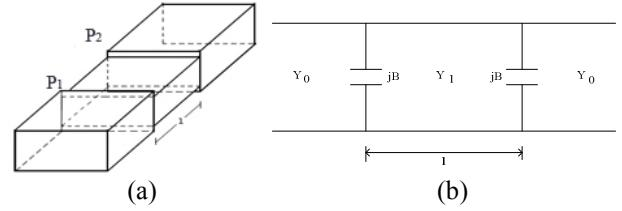
**Figure 4.** (a) Design model and (b) equivalent circuit of the mismatch waveguide section.
