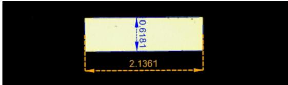
**Figure 8.** Waveguide aperture of the mismatch waveguide (VSWR2.0) seen through a microscope
