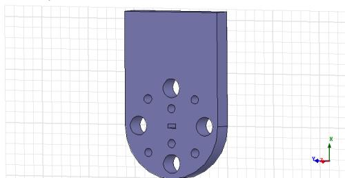
**Figure 3.** Machining model of the transmission phase standard.
