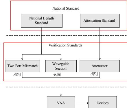
**Figure 1.** Traceability path of the 110GHz~170GHz S-parameter.
