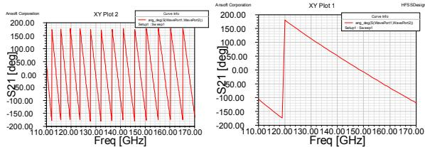
**Figure 2.** Simulation results of the match waveguide section with different length (left  $l=50\text{mm}$ , right  $l=3.822\text{mm}$ ).
