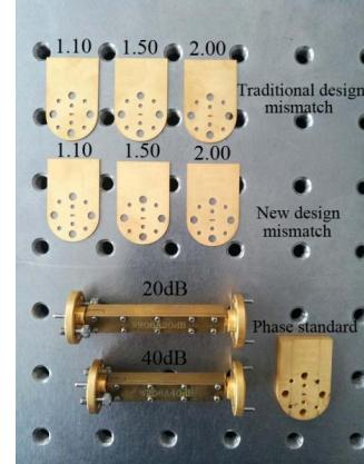
**Figure 7.** Photos of the processed verification standard.
