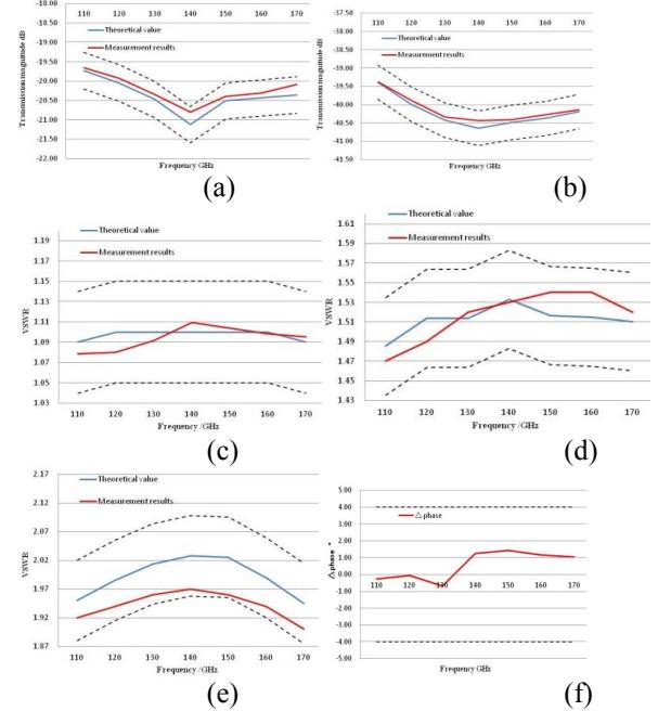
**Figure 10.** Results of system verification for VNA with (a)20dB attenuator ,(b)40dB attenuator,(c)1.10VSWR mismatch,(d)1.50VSWR mismatch, (e)2.00VSWR mismatch, and (f) $\Delta\phi$  of the match section.
