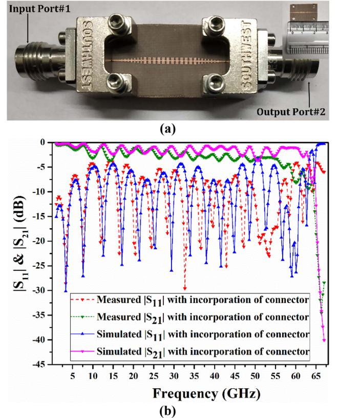
**Figure 4.** (a) Fabricated prototype of the proposed transmission line structure, (b) Magnitude of the simulated and measured reflection  $|S_{11}|$  and transmission coefficient  $|S_{21}|$ . [inset: size of the developed transmission line].
