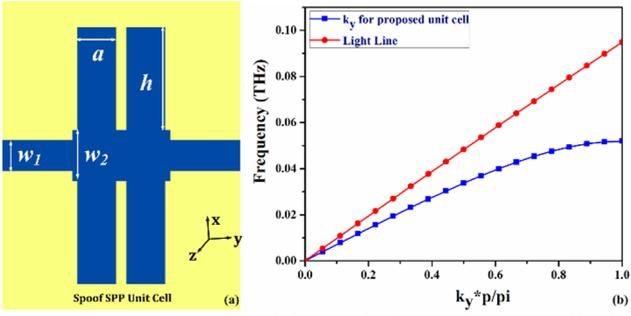
**Figure 1.** (a) Metamaterial spoof plasmonic unit cell, (b) dispersion curve.
