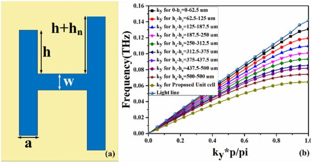
**Figure 2.** (a) Conversion and matching using gradient grooves, (b) dispersion curve.
