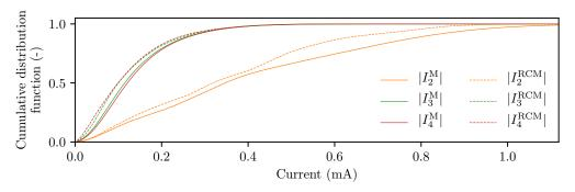
Figure 1. Comparison of CDF of induced current magnitudes computed from measurements and from simulation.
