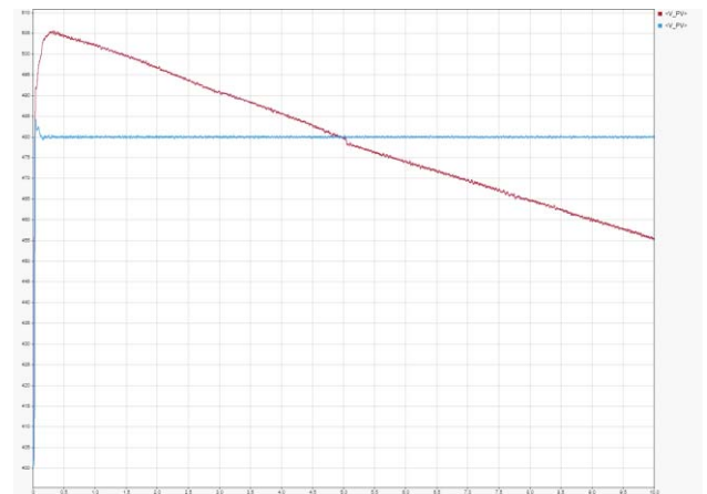
Figure 10. Voltage for temperature and irradiance growth (red plot – MPPT enabled, blue – MPPT disabled).
