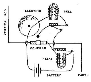
Figure 3. Popov's apparatus for the reception of radio disturbances. Note the essential circuit element ("coherer"), capable of changing itself into a conducting state when excited by an electric pulse from the antenna. The resulting current triggers electromagnets with the effect of a bell sound, followed by a knock on the coherer to bring it back into an insulating state.
