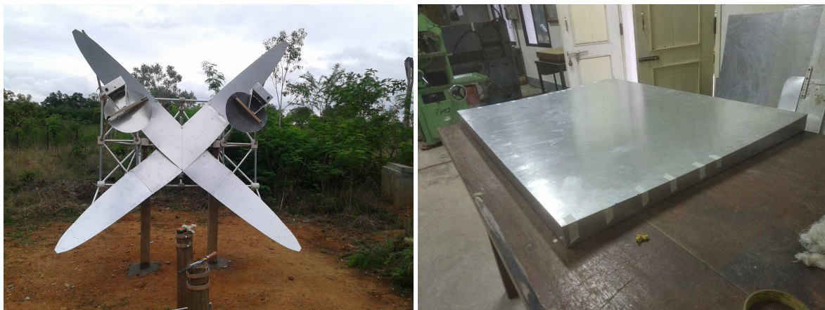
Figure 1. (a) Left picture is the 1/3 scaled-model of the RRI Efficient Linear-array Imager, being constructed at the Gauribidanur field-station. (b) Right picture shows the first prototype light-weight cylindrical panel made.
