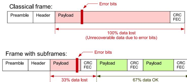
Figure 1. An explanation how the subframes can improve the total efficiency. In a case of bit errors in a classical frame, the whole payload has to be retransmitted. If the subframes are used, then only the invalid part is rejected and there is no need to retransmit the whole frame, only the defect part.
