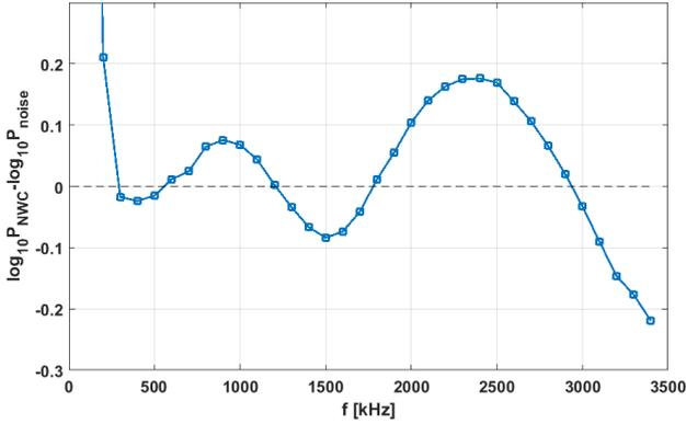
**Figure 1.** Variation of signal to noise ratio as a function of frequency. The signal is measured above NWC transmitter, noise is measured above the Pacific and Atlantic Oceans.
