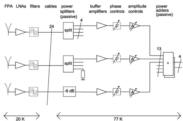
Figure 1. Block diagram of PHAROS front end.
