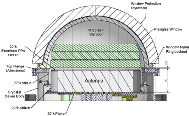
Figure 2. Drawing of vacuum window.
