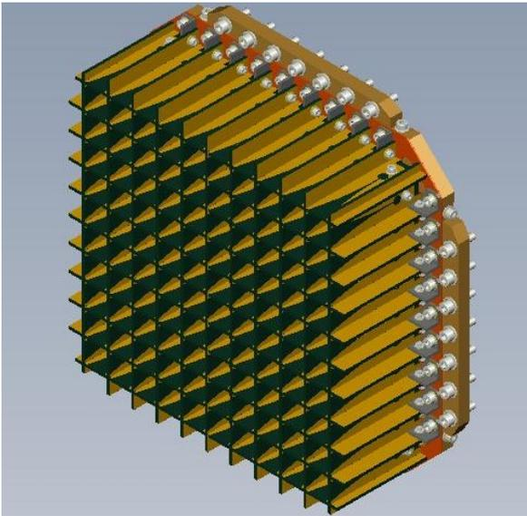
**Figure 5.** 3D drawing of PHAROS Vivaldi antenna array.
