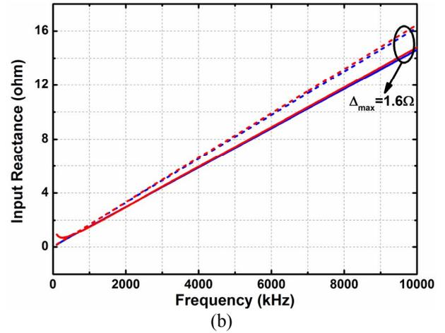
**Figure 5.** The measured (solid lines) and simulated (dash lines) (a) input resistance and (b) input reactance of the bar samples with fibers along (blue color) and across (red color) the length.
