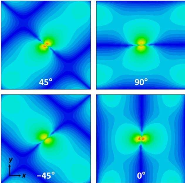
**Figure 7.** Distribution of current density of the top four layers of the 32-layer CFRP panel ( $45^\circ$ ,  $90^\circ$ ,  $-45^\circ$ , and  $0^\circ$  fiber orientations). The maximum magnitude denoted by red color is around  $2 \times 10^{11}$  A/m<sup>2</sup>.
