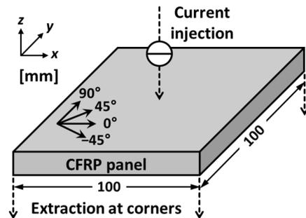
**Figure 6.** Lightning model for the 32-layer QI CFRP panel with the dimensions of 100 mm × 100 mm × 6.4 mm. Lightning current is injected at the center of the top surface and extracted at the four corners of the bottom surface.
