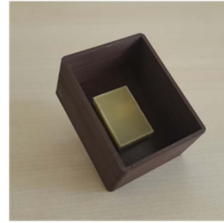
Figure 3. Patch antenna covered with two layers of FR4 superstrate mounted at the bottom of a 3D printed ABS container.
