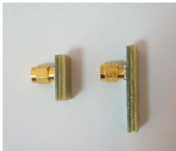
Figure 2. Patch antenna covered with two layers of FR4 superstrate mounted at the bottom of a 3D printed ABS container.
