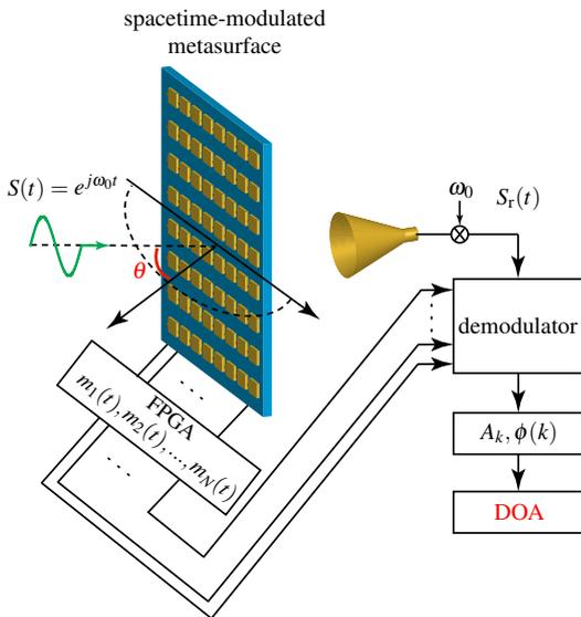
**Figure 2.** Direction-of-Arrival (DoA) estimation based on a spacetime-modulated metasurface [13].
