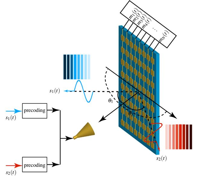
**Figure 3.** Spatial multiplexing based on a spacetime-modulated metasurface [15].
