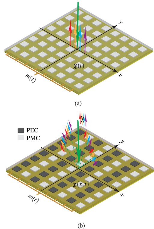
**Figure 1.** Camouflaging based on a spacetime-modulated metasurface [13]. (a) Time-only modulation, providing temporal spectrum spreading. (b) Spacetime modulation, providing simultaneously temporal and spatial spectrum spreading.
